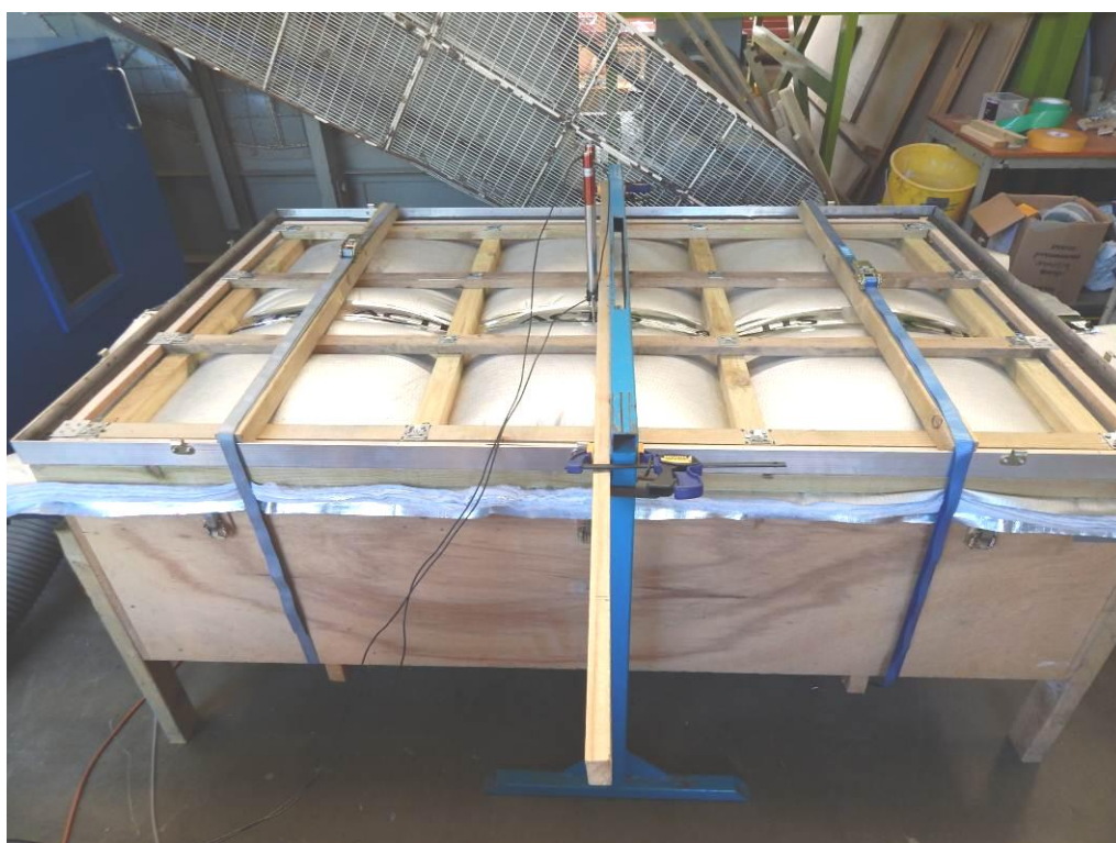
Figure 6 View of Boost'R Hybrid under test with taped laps at a batten at gauge of 345mm with 38mm counter battens
