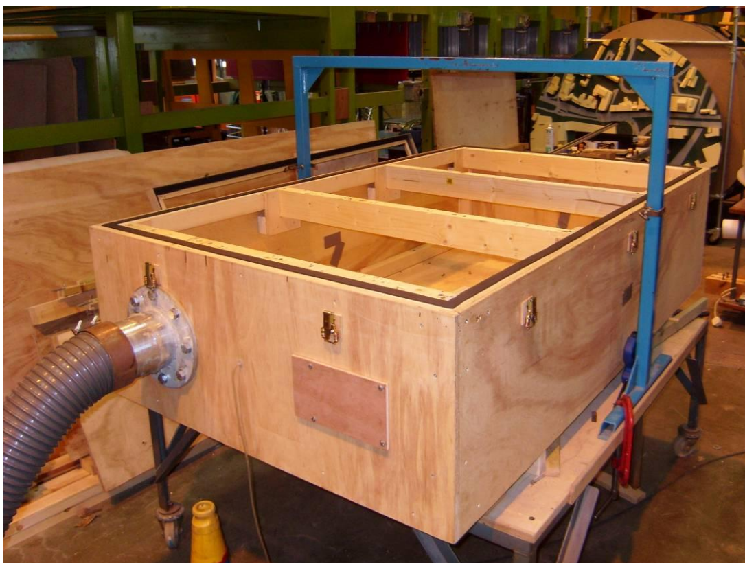
Figure 1 The BRE test chamber for Annex A tests
